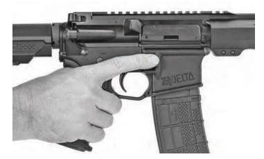
Hold the grip of the firearm while keeping your finger off the trigger. Press the magazine release button and pull the magazine down to remove.
