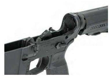
Warning: The buffer and action spring are under compression. Push down on the buffer retainer pin (A) while holding the buffer back. Allow buffer to travel forward slowly after clearing the retaining pin. Once the spring is no longer compressed, remove from buffer tube.
