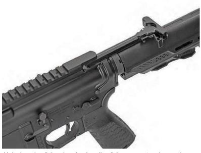
Unlock and pull the charging handle all the way out and press in on the lower portion of the bolt catch. Release charging handle. This locks the bolt in the open position.
