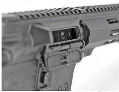
Look into the receiver through the ejection port and verify that there are no cartridges in the chamber.
