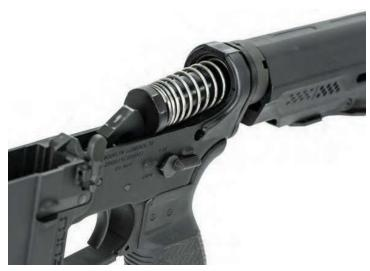
Clean inside of buffer tube with a cotton patch and CLP. Wipe down buffer and spring.
