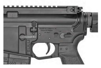
Place selector on SAFE and make sure rifle is pointed in a safe direction.
