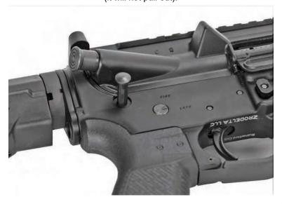
Grasp the rear of the upper receiver and pull up, allowing it to pivot on the front pin. This will expose the fire control group.
