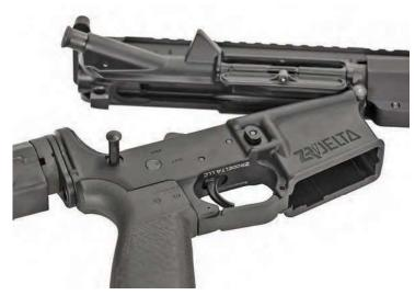
Unlatch the charging handle and pull it back. This will extract the bolt carrier group.
