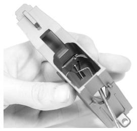
You can release the spring from the magazine catch by pulling it out of the recess with the screwdriver, hook, or with a pair of pliers (if needed).
