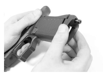
Once the bolt has been completely loosened, pull the magwell away from the frame. There should be a click as the hooks of the magwell disengage from the frame.
