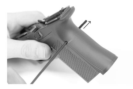
Press the trigger housing pin entirely out of the frame.
