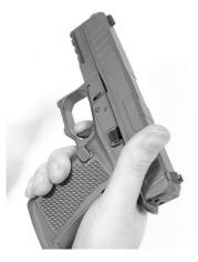
Ensure that the firearm is empty and pointed in a safe direction. Pull trigger all the way to the rear.
