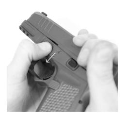
With the slide pulled slightly to the rear, pull the tabs of the slide lock down.
