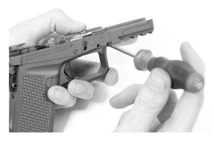
The second fastener is located on the side of the frame nearly in line with and toward the front of the trigger guard.
