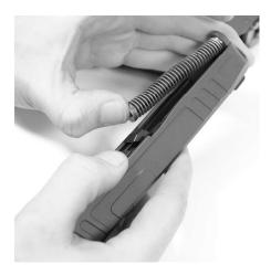
Compress the recoil spring assembly slightly forward and lift the rear away from the slide to remove the assembly.
