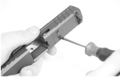
The slide plate is held into place by two bolts, located side by side on the top of the slide. Using the tool provided, unscrew and completely remove the two bolts.
