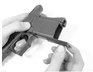
Once the magwell has been removed, the front strap will slide freely down from the frame.
