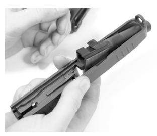
Remove barrel from the slide by slightly moving the barrel up and forward to clear the chamber of the barrel from the slide, then pulling barrel to rear.
