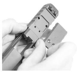
Once the bolts have been removed, pull the plate up away from the slide.
