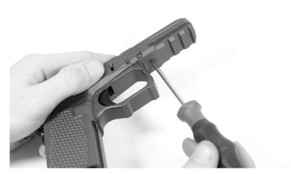
On the bottom side of the frame and dust cover, insert the bolt and tighten to 17 in-lbs. Do not clean off reusable thread locker present on this fastener.
