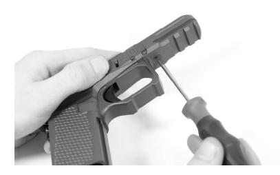
The first is located in front of the trigger guard on the bottom of the frame. With the tool provided, unscrew and completely remove the bolt. Do not clean off reusable thread locker present on this fastener.
