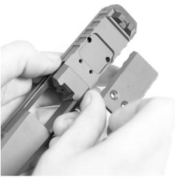
Ensure that the plate is properly orientated to the slide; the cut out and threaded bolt holes of the slide should line up with the holes and protrusion seen on the bottom of plate. Place the plate onto the slide so that the top is flush with the top of the slide. Insert and tighten the bolts to 6 in-lbs.
