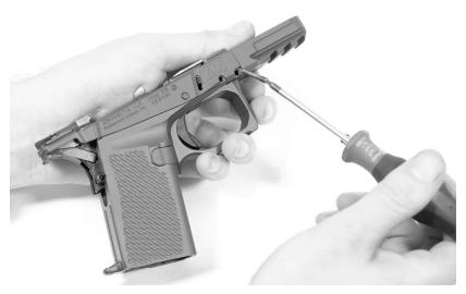
With the tool provided, unscrew and completely remove the threaded pin. Note: the threaded pin can only be removed from the right hand side of frame.
