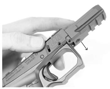
Push the dust cover down and slide the part off of the receiver.
