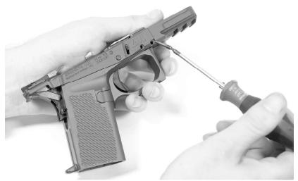
From the right hand side, insert the threaded pin and tighten to 10 in-lbs.
